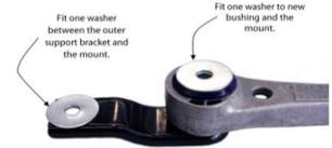
Fit one washer between the outer support bracket and the mount.
