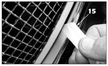
**15.** Carefully pull off the protective masking tape from around the upper grille surround. Pull the tape straight out to minimize tape breakage.
