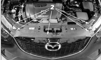
1. Open the hood and use a flat blade screwdriver to remove the plastic push pins securing the center poriton of the radiator support panel cover. Once the push pins have been removed, slide the panel forward to remove it.
