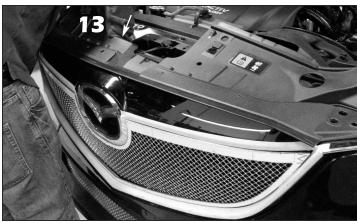
**13.** Reach down from underneath the radiator suport panel and install the supplied small black plastic washers and #8-32 ESNA half nuts to the studs across the sides and bottom of the mesh grille. Install the supplied large black plastic washers and #8-32 ESNA half nuts onto the studs across the top of the grille.
