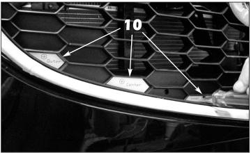
**10**. Cut out and align the supplied hole location templates and tape them into place. Use an awl or similar pointed tool top mark the hole locations onto the factory grille. Untape the templates, flip them over and mark the opposite side.
