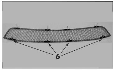
**6.** Install the supplied black cap plugs over the lower four (4) studs after the closed ends have been trimmed off.
