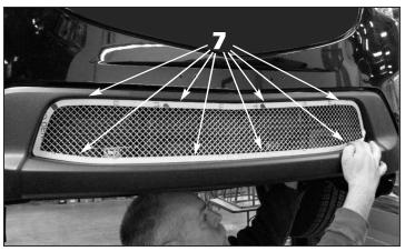
**7**. Carefully align the lower grille into place, making sure that the studs pass through the openings in the factory grille.
